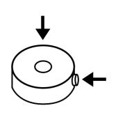
Two options for cable gland installation: at the top or at the side
